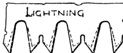
FIG. 8.—TEETH OF LIGHTNING SAW.
